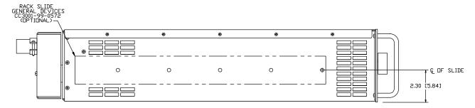
Figure 3-1: Rack Mount Slides (-RMS option) position
