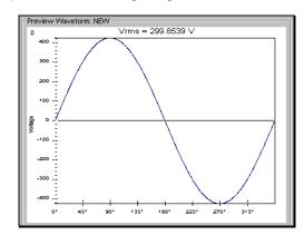
Figure 4-9: Waveform Crest Factor Affects Max. rms Voltage
