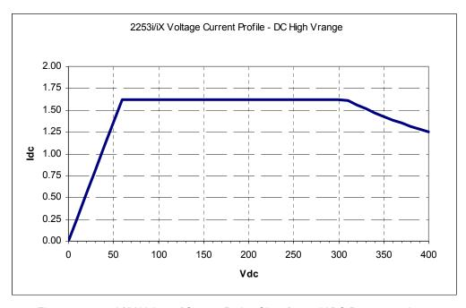
Figure 2-6: 2253i / iX Voltage / Current Rating Chart for 400V DC Range per phase.
