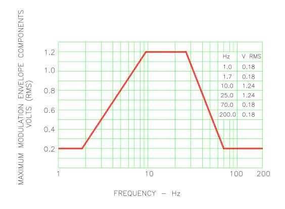
Figure 9-4: Voltage Modulation - Frequency characteristics
