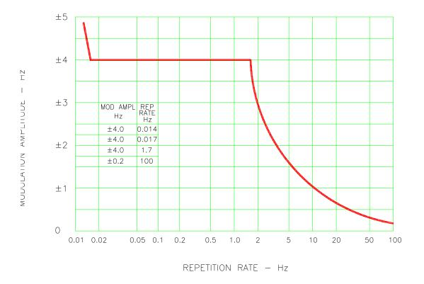
Figure 9-5: Frequency Modulation
