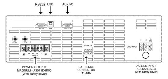
Figure 3-2: Rear Panel Connector Locations – i Models
