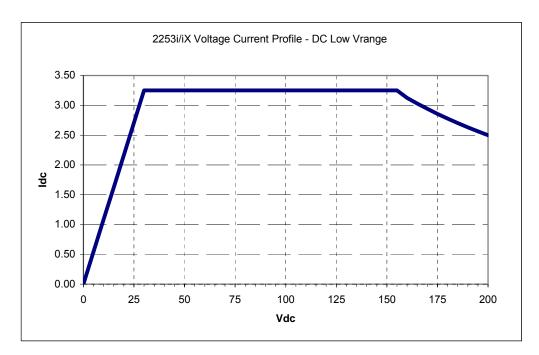
Figure 2-5: 2253i / iX Voltage / Current Rating Chart for 200V DC Range per phase.
