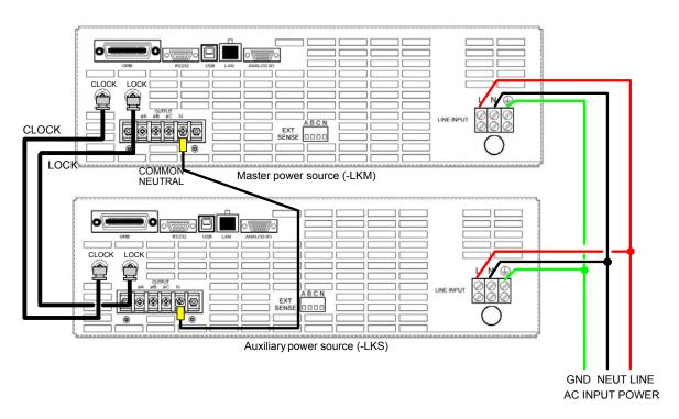
Figure 3-6: Clock and Lock Connections
