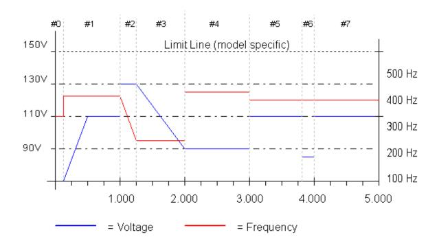
Figure 4-12: Sample Transient Output Sequence
