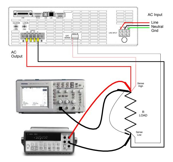
Figure 3-5: Functional Test Setup
